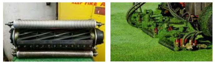
**Figure 6-3.** Reel mowers are used on greens, collars, tees, approaches, and fairways. Proper reel to bed knife adjustment is necessary to maintain plant health. Photos from New England Regional Manual.
