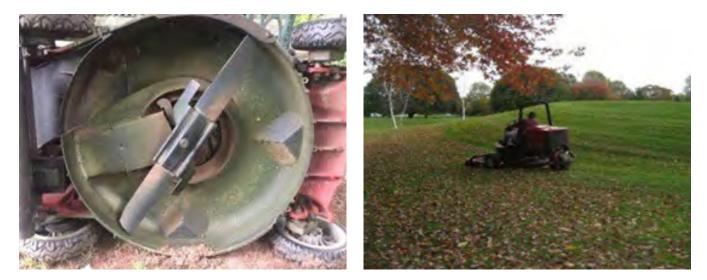
**Figure 6-4.** Rotary mowers are used for rough and surrounds (bunker, green, and tee). Sharp rotary blades are necessary for a quality cut and plant health. Photos from New England Regional Manual.
